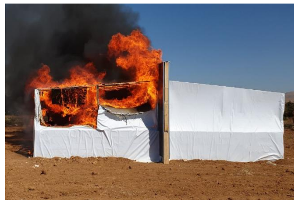
Figure 3 – Illustration of partition wall installed between two back to back shelters
