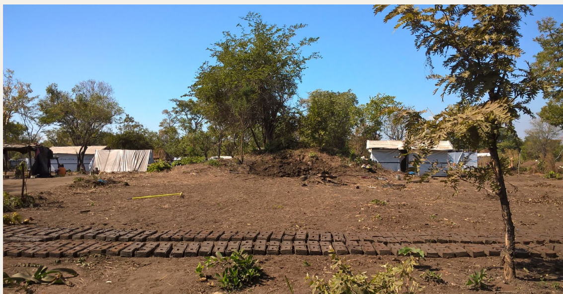
Sun dried bricks produced by a family, Dombe, 2019 Source: Sonia Molina
