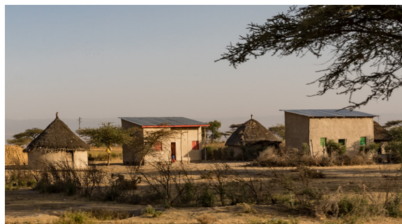
Rectangular houses with CGI sheet roofs and round houses with thatched roofs, both with chikka walls near Langan lake, Oromia. CC- Nina
