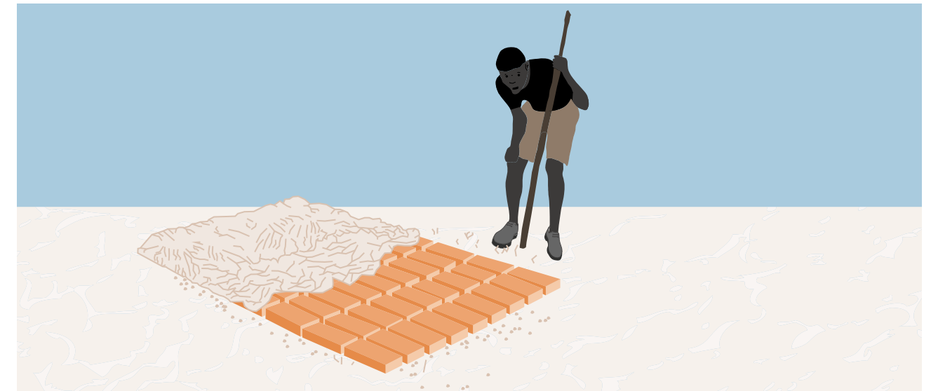
18. BRICK CURING UNDER GRASS/ STRAW
