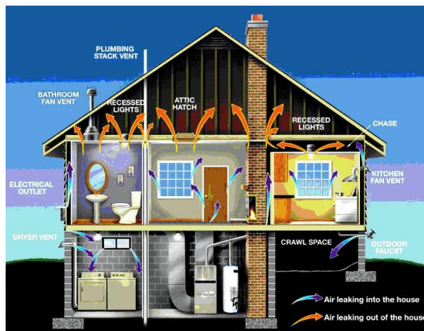
Figure 33 Classic air leak affecting insulation performance
