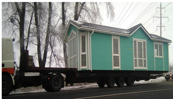
Figure 13 example of prefabrication, 45 sqr meter, 10,000 USD. The unit is transported as a full house and set up with a crane Dobraya Vest 2016
